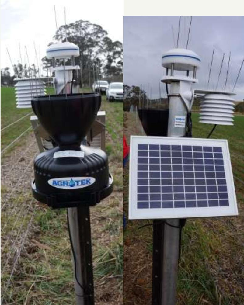
Photos above show weather station & moisture probes. They are solar & battery powered.
